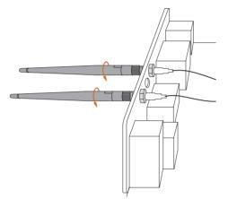
7. Set the WiFi 2.4/5/6 GHz Antennas at 90-degree angle. \*You may need to adjust the direction of the antenna for a stronger signal.
