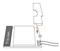
4. Insert the two RF cables into the antenna ports on the I/O shield.
