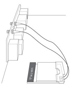
5. Secure the RF cables with the bundled screw nuts and washers.
