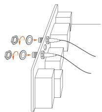
Connect the two WiFi 2.4/5/6 GHz Antennas to the antenna connectors. 6. Turn the antenna clockwise until it is securely connected.
